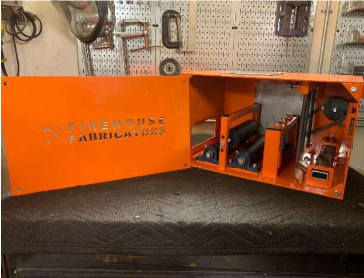
These machinery extrication props are able to be cut, pried, and disassembled, allowing for more realistic training.
